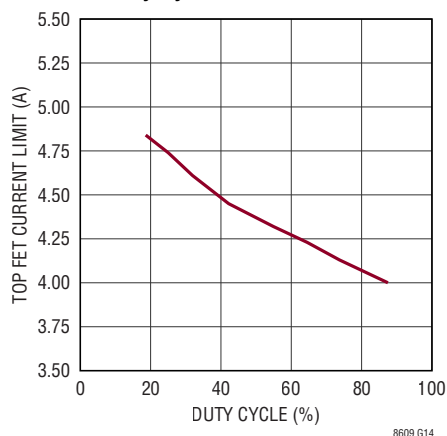
Top FET Current Limit vs Duty Cycle
