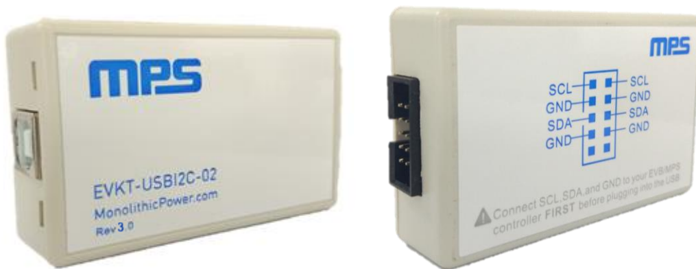
Figure 2: EVKT-USBI2C-02 Communication Interface
