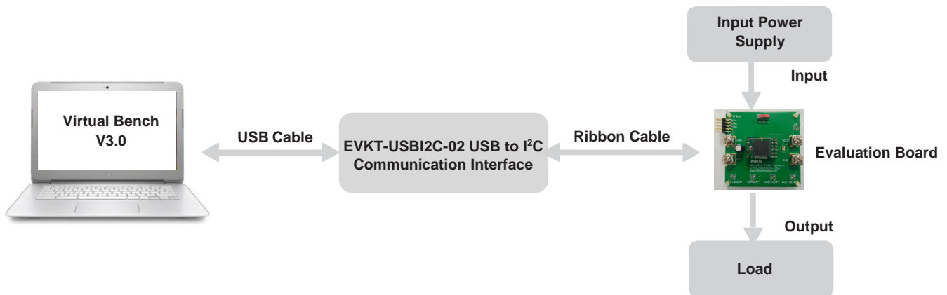
Figure 1: PKT-mEZDPD1620A Evaluation Kit Set-Up
