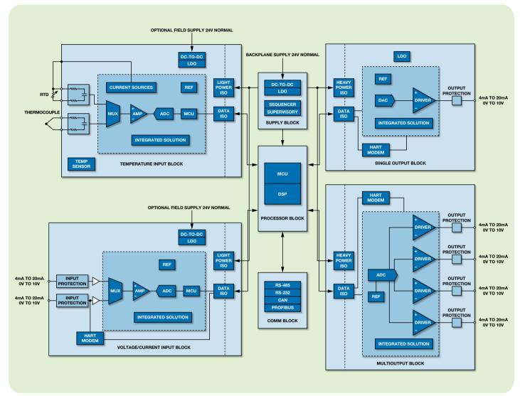
Note: the signal chains above are representative of a PLC application system. The technical requirements of the blocks vary, but the products listed in the table are representative of ADI's solutions that meet some of those requirements.
