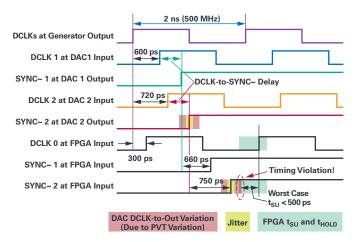
Figure 11. Subclass 2 multiple DAC application SYNC~/DCLK timing violation.
