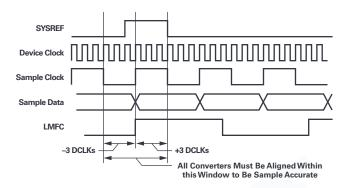
Figure 7. Sample accurate requirement for SYSREF capture.
