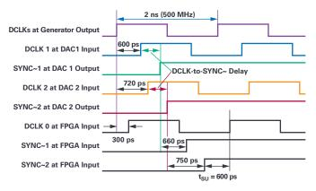
Figure 10. Subclass 2 multiple DAC application SYNC~/DCLK timing.
