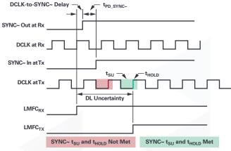
Figure 13. Subclass 2 SYNC~ capture timing for a single converter application: worst case DLU.
