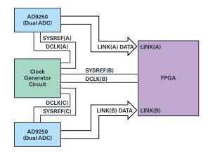
Figure 3. SYSREF/DCLK routing for a 3-device JESD204B system.
