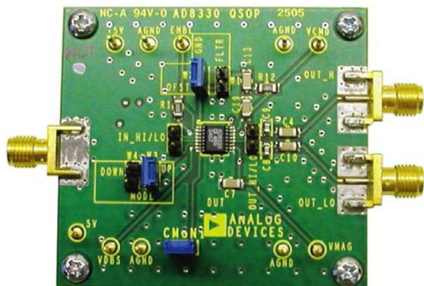
Figure 1. Photograph of the AD8330 Evaluation Board
