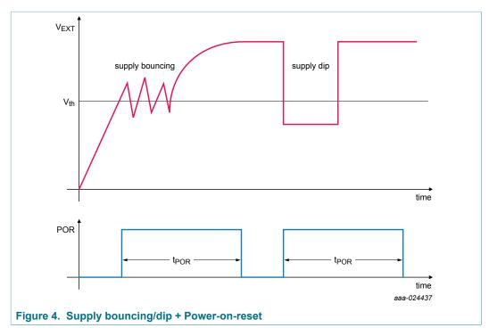
When  $V_{EXT}$  drops below  $V_{POR}$ , the power-on reset circuit drives the RESETN signal LOW weakly to generate a clean reset signal to reset the PMU. The PMU prolongs the reset for  $t_{POR}$  to reset the rest of the chip. When not active, the power-on reset circuit is driving the RESETN signal weakly HIGH (see Figure 5).
