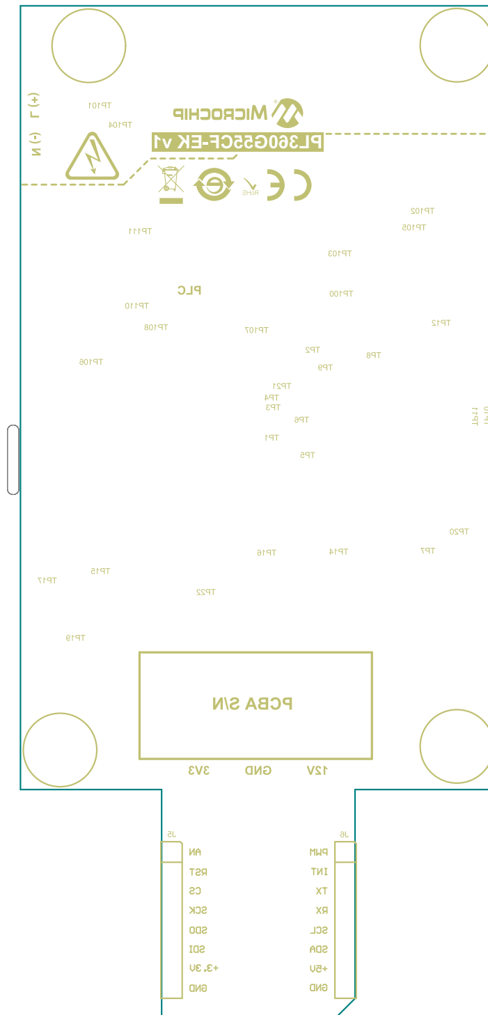
Figure 3-33. PL360G55CF-EKv1 Layout: Bottom Silkscreen
