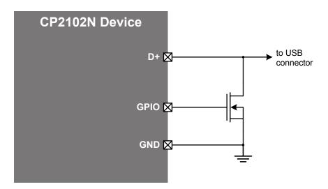
This circuit uses an NMOS transitor and a GPIO pin to short D+ to ground during power-on. The GPIO pin will be open drain and pulled high through a weak pull-up during reset. The GPIO should be configured so that the [Reset Latch] value is [Low], which turns off the transistor after reset and enables the device to enumerate normally. GPIO can be configured using Xpress Configurator in Simplicity Studio v4 (www.silabs.com/simplicity).
