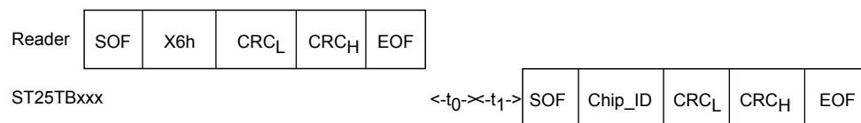
Figure 49. Slot_marker frame exchange between reader and ST25TB04K
