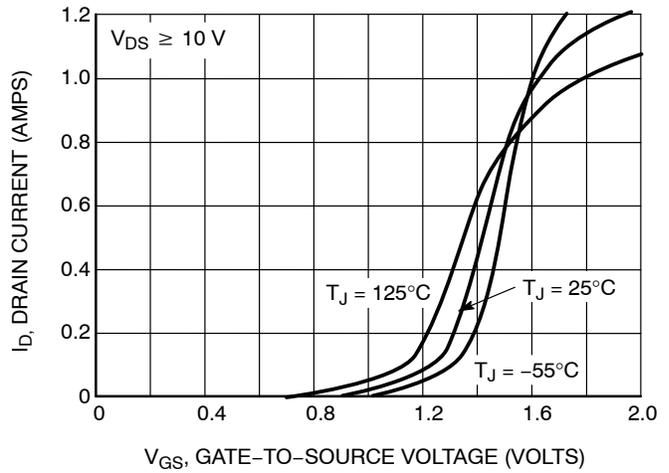
Figure 2. Transfer Characteristics
