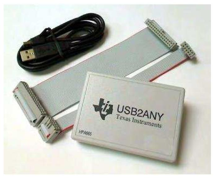
Figure 5. USB2ANY Box and Cables
