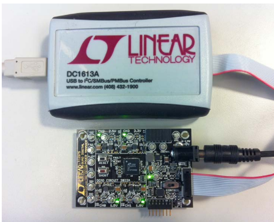
Figure 2. Connecting DC2022A Board and the DC1613 I 2 C/SMBus/PMBus Controller
