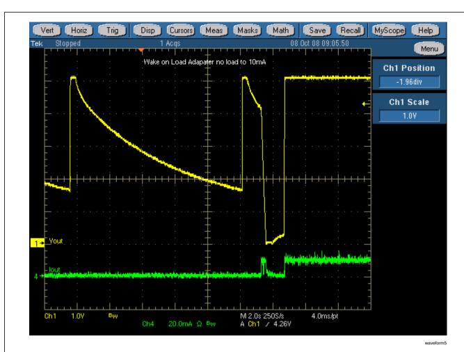
FIGURE 9. Change from no load to 10ma load at 100 VDC input
