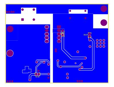
FIGURE 13. PCB Layout Bottom, as viewed from the bottom
