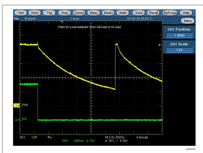
FIGURE 7. Change from full load to no load at 100 VDC input
