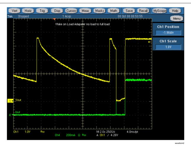
FIGURE 6. Change from no load to full load at 100VDC input
