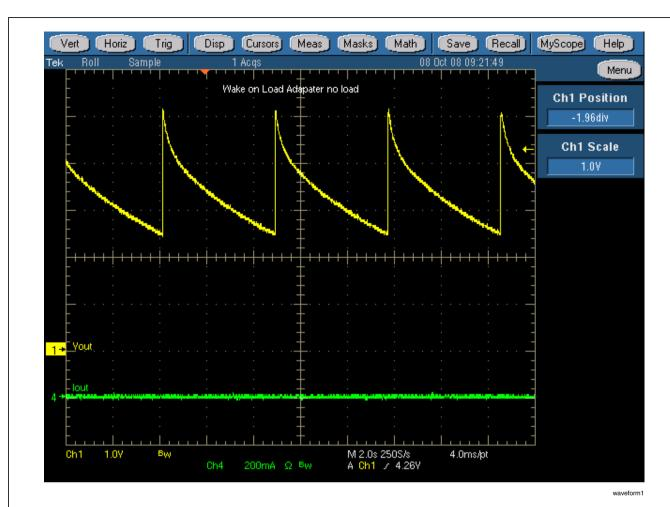
FIGURE 5. No Load Operation at 339 VDC input
