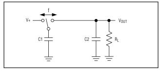
Figure 3a. Switched-Capacitor Model
