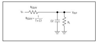
Figure 3b. Equivalent Circuit
