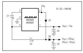
Figure 6. Combined Doubler and Inverter
