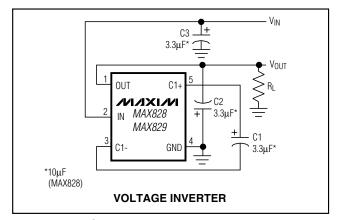
Figure 1. Test Circuit
