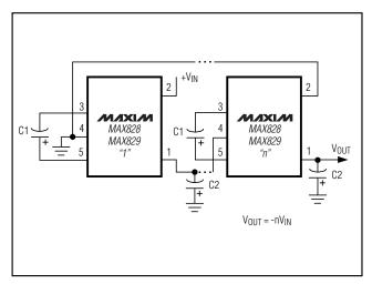
Figure 4. Cascading MAX828s or MAX829s to Increase Output Voltage
