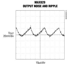
$V_{IN}$  = 3.3V,  $V_{OUT}$  = -3.2V,  $I_{OUT}$  = 5mA, AC COUPLED
