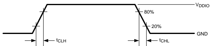
Figure 1. LVC MOS Transition Times
