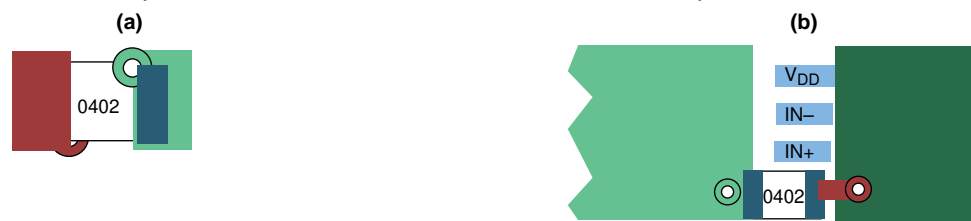
Figure 28. Typical Decoupling Capacitor Layouts
