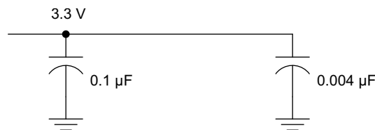
Figure 17. Recommended M-LVDS Bypass Capacitor Layout
