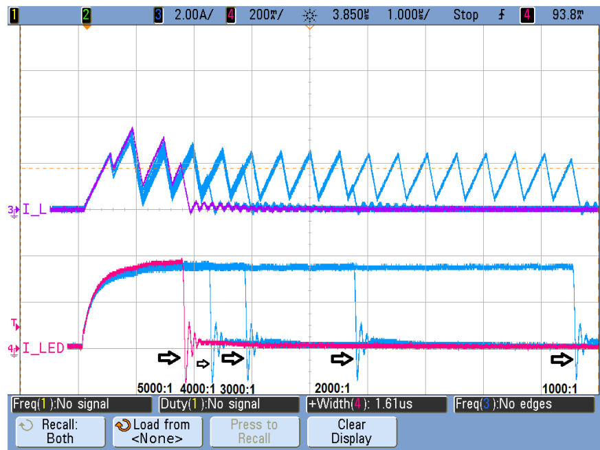
Figure 2. DC2361A 12VIN 120Hz PWM Dimming Waveforms at Different PWM Duty Cycles with 5000:1 in Bold. I_{LED} Waveform (200mA/Div) Is on the Bottom (with 40V LED String) and I_L Waveform (2A/Div) Is on the Top.
