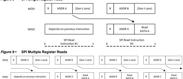
The SPI read instruction figures also point out the read/write state and address bits on the MISO output match the information received in the previous instruction. The SPI master could use this data to verify the device captured the previous instruction properly, or simply ignore the data. The following illustration shows the MISO output during write instructions reporting the previous instruction's read/write state, address, and register write data.
