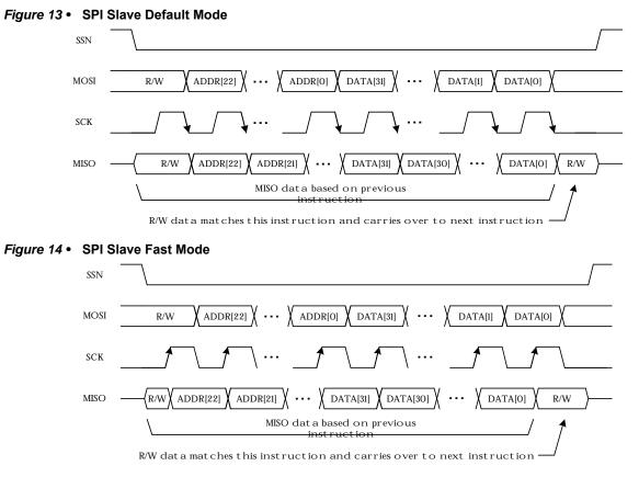
MISO output timing is the only difference between the two SPI modes. Sampling of MOSI on the rising SCK clock edge remains the same so writing to the VSC8256-01 device registers is identical in both modes. Thus the SPI\_CTRL.FAST\_MODE register setting may be modified using the SPI slave port to change the port's MISO output timing.
