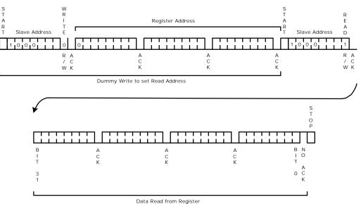
The two-wire serial slave interface supports sequential read and sequential write instructions.
