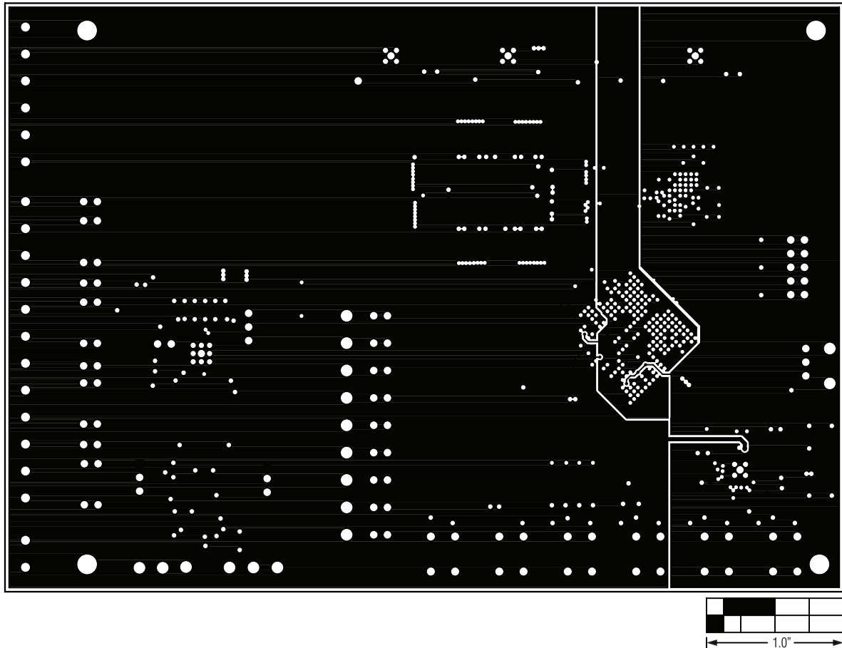
Figure 17. MAX11043 EV Kit PCB Layout—Signal Layer 6
