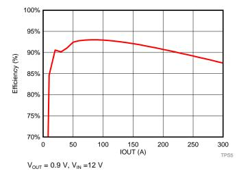
Figure 12. VOUT A Power Stage Efficiency
