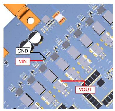
Figure 11. Test Setup for Efficiency Measurement
