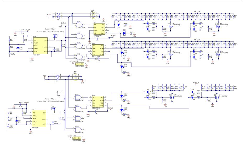
Figure 8. TPS53681EVM - On Board Transient Load Schematic
