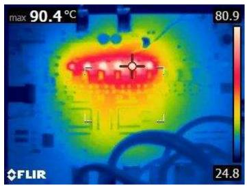
A  $V_{IN} = 12 \text{ V}, V_{OUT} = 0.9 \text{ V}, I_{OUT} = 294 \text{A}$
