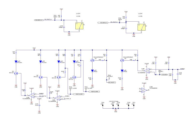
Figure 6. TPS53681EVM - Helper Circuits and Indicators Schematic
