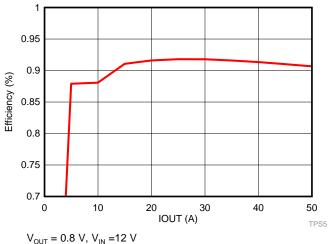
Figure 13. VOUT B Power Stage Efficiency
