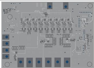
Figure 31. Bottom Layer Assembly Drawing (Bottom View)
