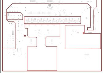
Figure 35. Internal Layer 3 (Top View)
