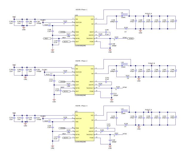
Figure 4. TPS53681EVM - Rail B Power Stages Schematic
