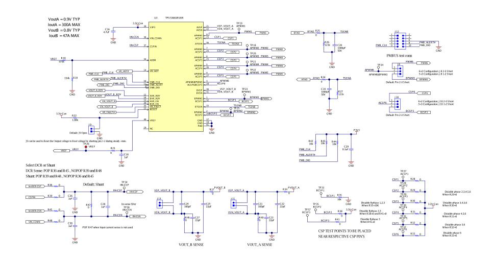
Figure 1. TPS53681EVM - Controller Schematic
