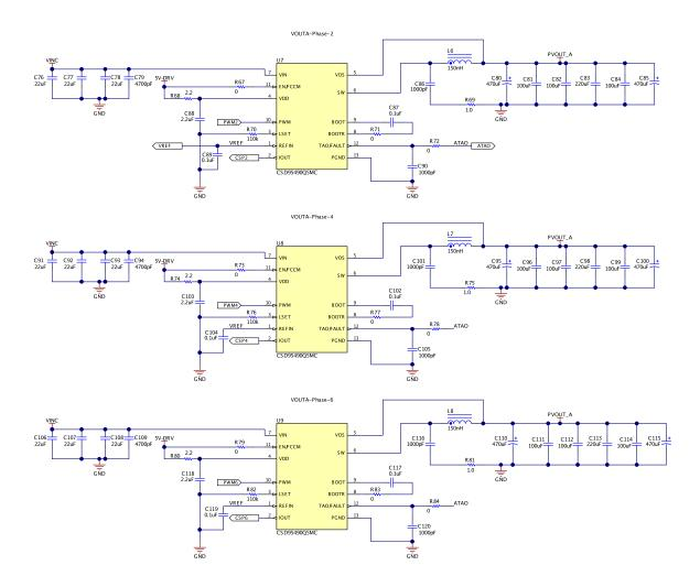
Figure 3. TPS53681EVM - Rail A Power Stages 2-4-6 Schematic
