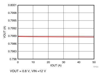
Figure 15. VOUT B Load Regulation
