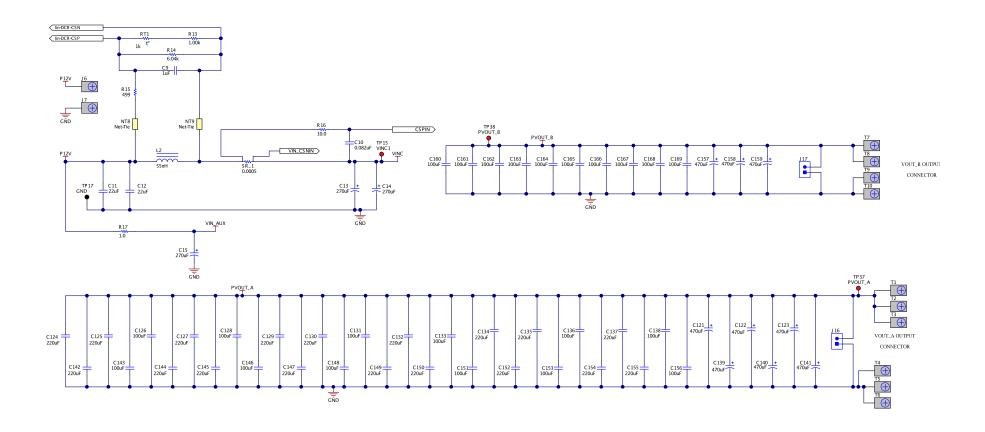
Figure 7. TPS53681EVM - Input and Output Filter Schematic
