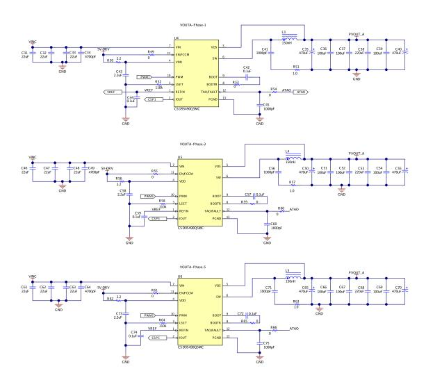
Figure 2. TPS53681EVM - Rail A Power Stages 1-3-5 Schematic
