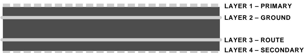
Figure 4. Four Layer Stackup
