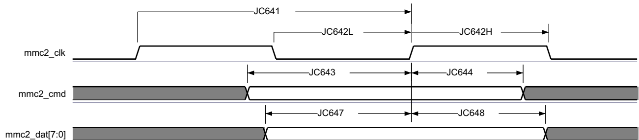
Figure 7-76. MMC/SD/SDIO in - High Speed JC64 - Receiver Mode
