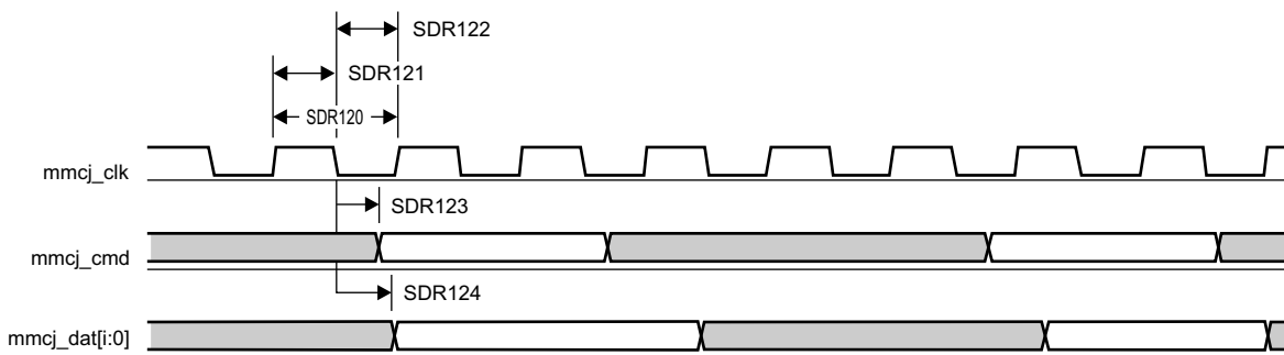
Figure 7-86. MMC/SD/SDIOj in - SDR12 - Transmitter Mode
