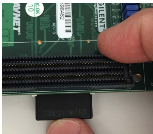
Figure 3. Inserting the SD card into the ZedBoard.
