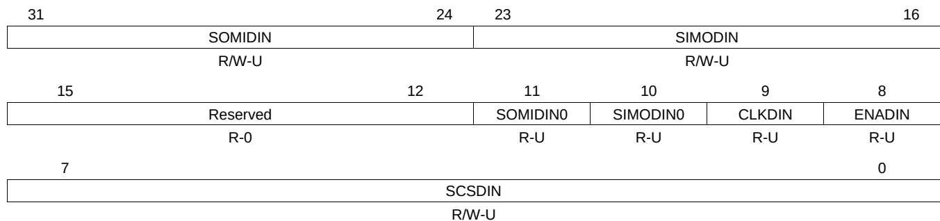
Figure 25-33. SPI Pin Control Register 2 (SPIPC2) [offset = 1Ch]
