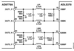
Figure 3. DAC Modulator Interface with 3 MHz Third-Order, Elliptical Low-Pass Filter (Calculated Component Values)
