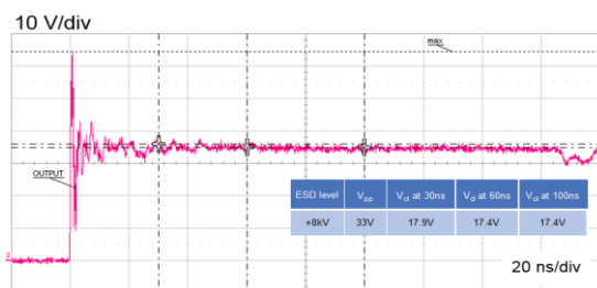
Figure 7: ESD response to IEC 61000-4-2 (+8kV contact discharge)
