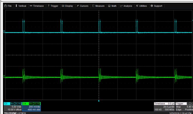
Figure 16. LPM Mode Operation (when a burst packet contains 2 pulses and the interval between 2 packets is around 40µs, and peak current starts to reduce. CH3 = PWML, CH4 = Transformer primary winding current.)
