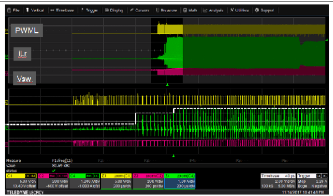
Figure 15. Recovery after OPP with 3 Stages of Peak Current (CH1 = PWML, CH4 = Transformer Primary Winding Current, CH2 = Switch Node Voltage)
