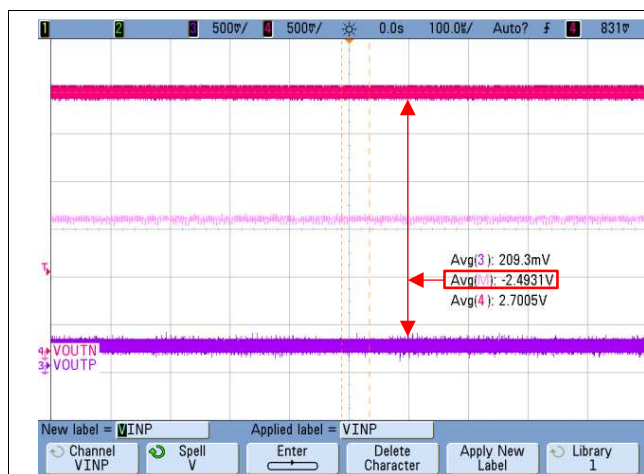
Figure 50. Typical Negative Clipping Output of the AMC1302
