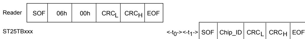
Figure 18. Initiate frame exchange between reader and ST25TB512-AT
