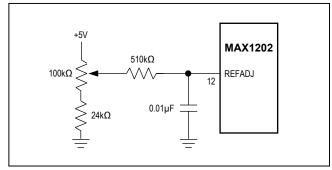
Figure 17. MAX1202 Reference-Adjust Circuit
