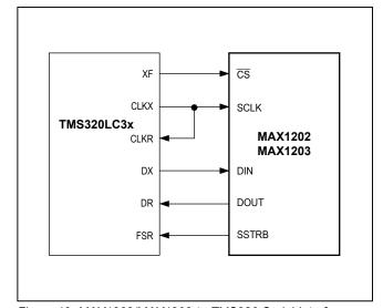
Figure 19. MAX1202/MAX1203-to-TMS320 Serial Interface
