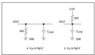
Figure 2. Load Circuits for Disable Time
