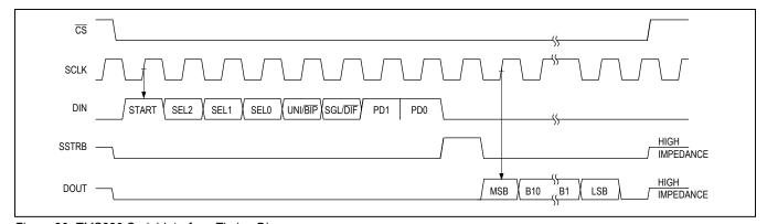
Figure 20. TMS320 Serial-Interface Timing Diagram
