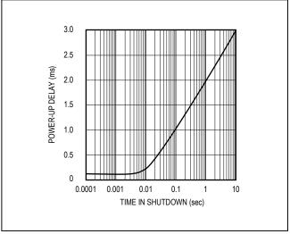
Figure 14c. Typical Power-Up Delay vs. Time in Shutdown
