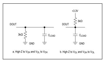
Figure 1. Load Circuits for Enable Time
