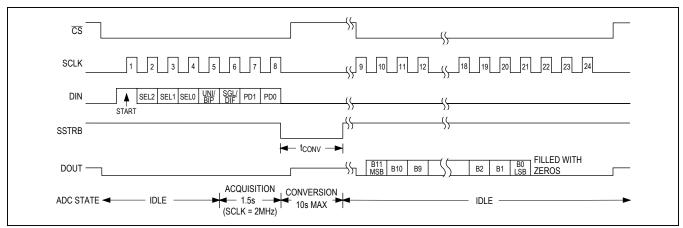
Figure 9. Internal Clock Mode Timing
