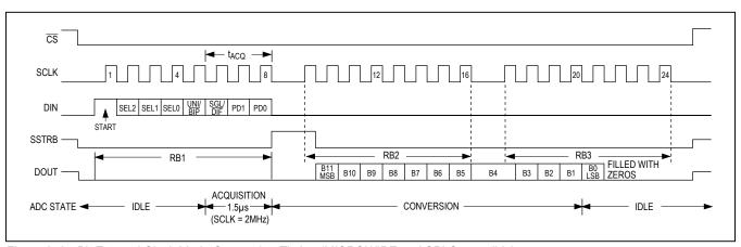
Figure 6. 24-Bit External Clock Mode Conversion Timing (MICROWIRE and SPI Compatible)
