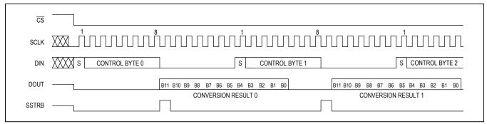
Figure 11a. External Clock Mode, 15 Clocks/Conversion Timing
