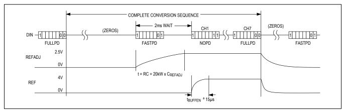
Figure 13. MAX1202 FULLPD/FASTPD Power-Up Sequence
