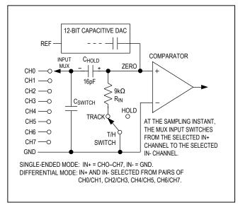
Figure 4. Equivalent Input Circuit
