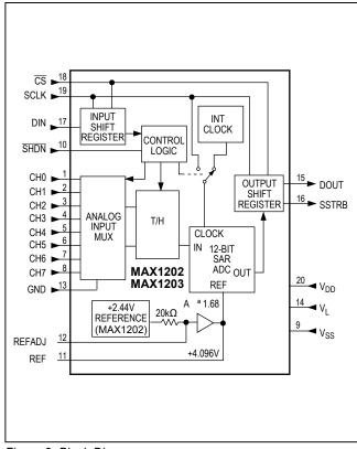
Figure 3. Block Diagram
