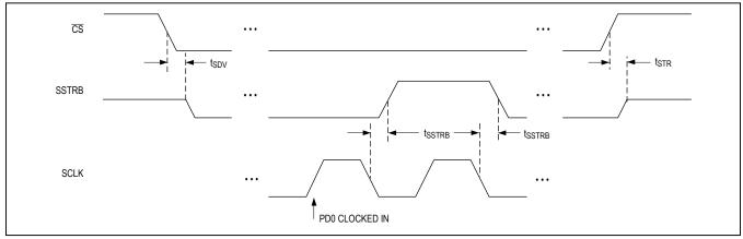
Figure 8. External Clock Mode SSTRB Detailed Timing
