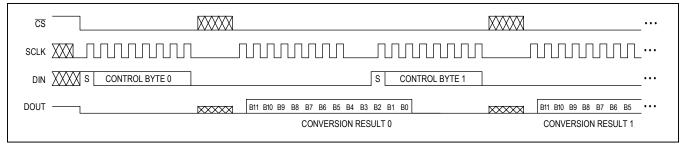
Figure 11b. External Clock Mode, 16 Clocks/Conversion Timing
