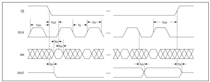
Figure 7. Detailed Serial-Interface Timing
