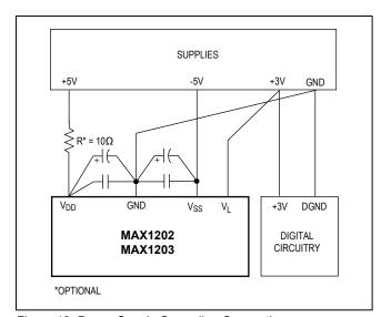
Figure 18. Power-Supply Grounding Connection
