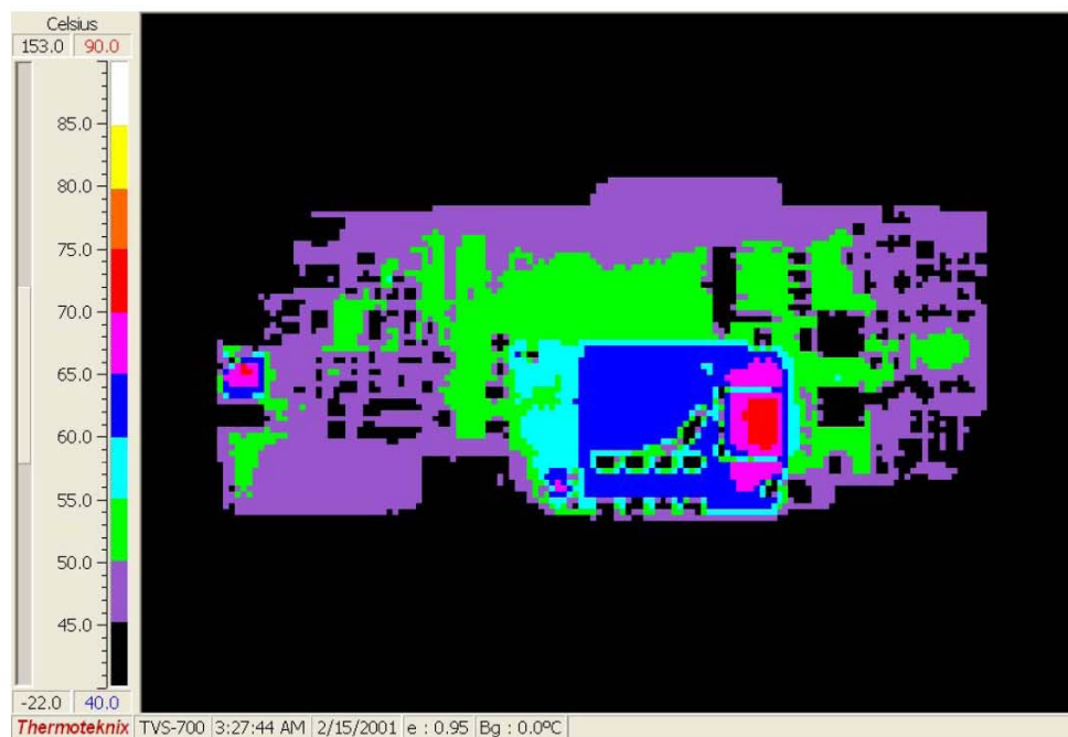
Figure 7. Thermal Map, Backside at 18Vin and 10Aout (Ta = 25 degrees C)
