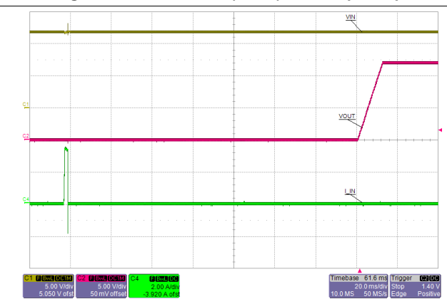
TPS25926x, V_{IN} = 12\text{ V} , C_{dVdT} = 1\text{ nF}
