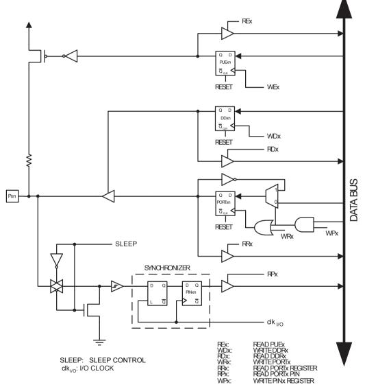
**Note:** WEx, WRx, WPx, WDx, REx, RRx, RPx, and RDx are common to all pins within the same port.  $clk_{I/O}$ , SLEEP are common to all ports.
