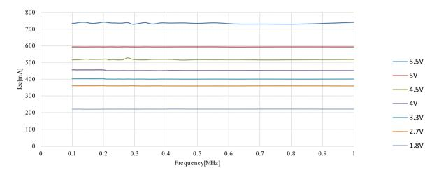
**Note:** The default clock source for the device is always the internal 8 MHz oscillator. Hence, current consumption in reset remains unaffected by external clock signals.
