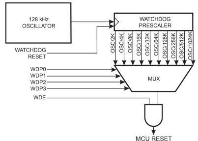
The Watchdog Timer can also be configured to generate an interrupt instead of a reset. This can be very helpful when using the Watchdog to wake-up from Power-down.
