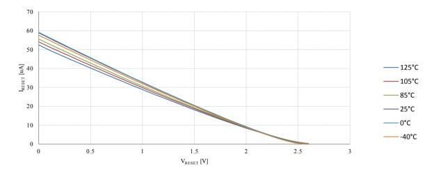
Figure 23-35. Reset Pull-up Resistor Current vs. Reset Pin Voltage (V<sub>CC</sub> = 5V)
