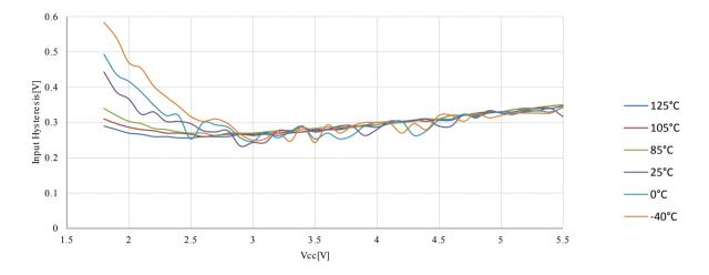
Figure 23-23. Reset Pin as I/O, Input Threshold Voltage vs.  $V_{CC}$  (V<sub>IH</sub>, I/O Pin Read as '1')
