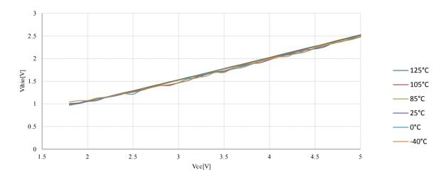
Figure 23-21. I/O Pin Input threshold Voltage vs.  $V_{CC}$  (V<sub>IL</sub>, IO Pin Read as '0')
