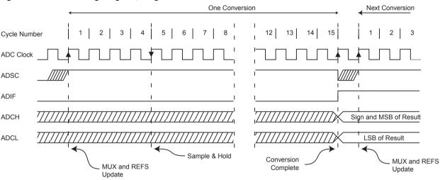
Figure 19-5. ADC Timing Diagram, Single Conversion
