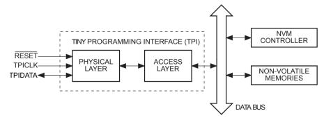
Programming is done via the physical interface. This is a 3-pin interface, which uses the RESET pin as enable, the TPICLK pin as the clock input, and the TPIDATA pin as data input and output. NVM can be programmed between 1.8-5.5V.
