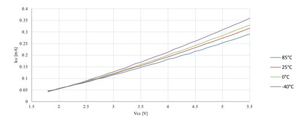
Figure 23-49. Watchdog Timer Current vs. V<sub>CC</sub>
