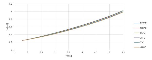
Figure 23-9. Idle Supply Current vs. V<sub>CC</sub> (Internal Oscillator, 1 MHz)
