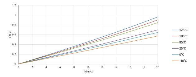
Figure 23-15. I/O Pin Output Voltage vs. Source Current (V<sub>CC</sub> = 1.8V)
