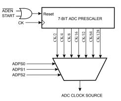
When initiating a single ended conversion by writing a '1' to the ADC Start Conversion bit (ADCSRA.ADSC), the conversion starts at the following rising edge of the ADC clock cycle.
