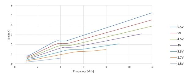
Figure 23-3. Active Supply Current vs. V<sub>CC</sub> (Internal Oscillator, 8 MHz)
