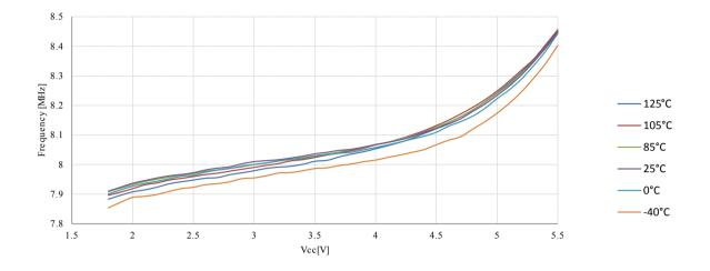
Figure 23-39. Calibrated Oscillator Frequency vs. Temperature
