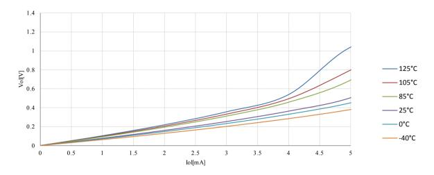
Figure 23-13. I/O Pin Output Voltage vs. Sink Current (V<sub>CC</sub> = 3V)
