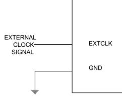
When applying an external clock, it is required to avoid sudden changes in the applied clock frequency to ensure stable operation of the MCU. A variation in frequency of more than 2% from one clock cycle to the next can lead to unpredictable behavior. It is required to ensure that the MCU is kept in Reset during the changes.
