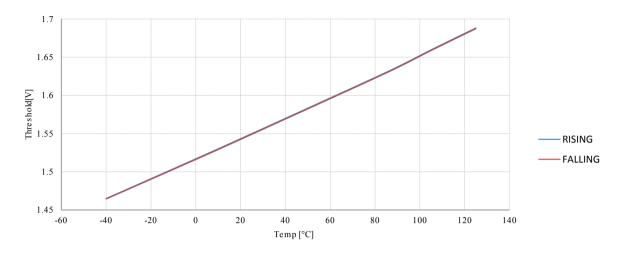
Figure 23-43. VLM2 Threshold of  $V_{CC}$  Level Monitor
