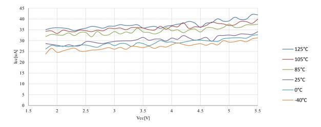
Figure 23-47. V<sub>CC</sub> Level Monitor Current vs. V<sub>CC</sub>
