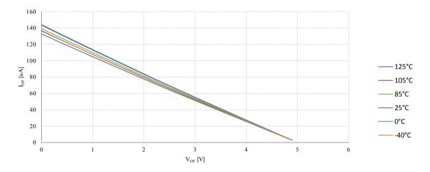
Figure 23-33. Reset Pull-up Resistor Current vs. Reset Pin Voltage (V<sub>CC</sub> = 1.8V)
