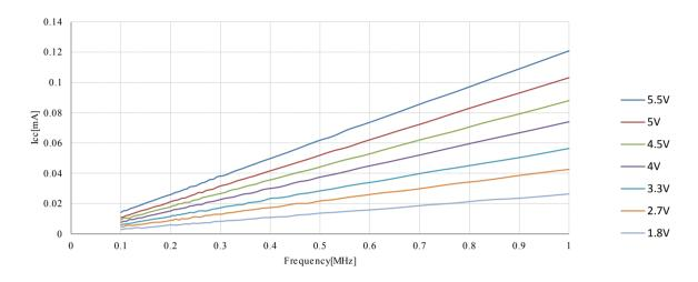
Figure 23-7. Idle Supply Current vs. Frequency (1 - 12 MHz)
