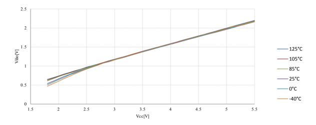
Figure 23-25. Reset Input Hysteresis vs.  $V_{CC}$  (Reset Pin Used as I/O)
