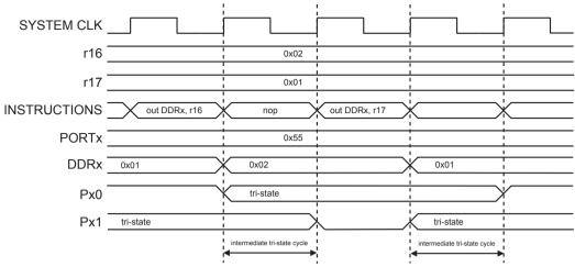
Figure 14-3. Switching Between Input and Output in Break-Before-Make-Mode
