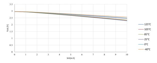
Figure 23-17. I/O Pin output Voltage vs. Source Current (V<sub>CC</sub> = 5V)
