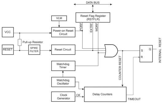
The I/O ports of the AVR are immediately reset to their initial state when a reset source goes active. This does not require any clock source to be running.
