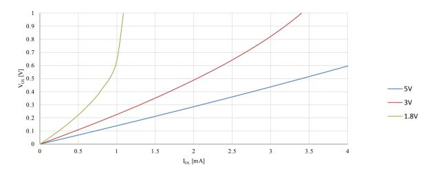
Figure 23-19. Reset Pin as I/O, Output Voltage vs. Source Current
