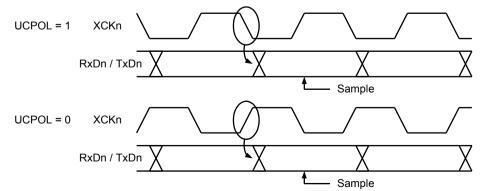
The UCPOL bit UCRSC selects which XCKn clock edge is used for data sampling and which is used for data change. As the above timing diagram shows, when UCPOL is zero, the data will be changed at
