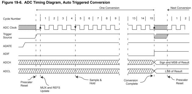
In Free Running mode, a new conversion will be started immediately after the conversion completes, while ADCRSA.ADSC remains high. See also the ADC Conversion Time table below.
