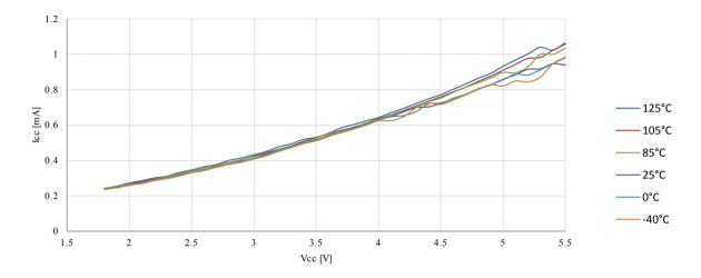
Figure 23-5. Active Supply Current vs.  $V_{CC}$  (Internal Oscillator, 128 kHz)
