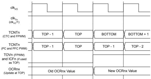
Figure 17-14. Timer/Counter Timing Diagram, no Prescaling.
