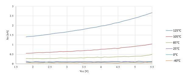
Figure 23-11. Power-down Supply Current vs. V<sub>CC</sub> (Watchdog Timer Enabled)
