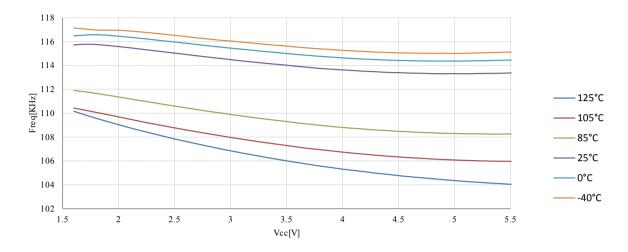
Figure 23-37. Watchdog Oscillator Frequency vs. Temperature
