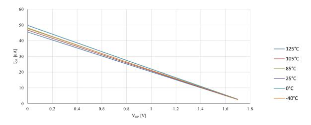
Figure 23-31. I/O Pin Pull-up Resistor Current vs. input Voltage (V<sub>CC</sub> = 2.7V)
