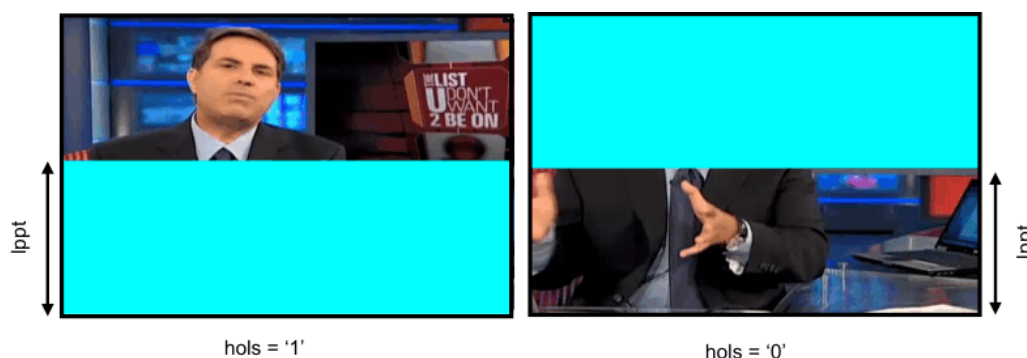
Figure 26-15. Subpicture Output with HOLDS Bit Variations
