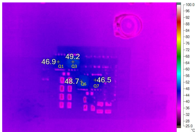
Figure 7. Thermal performance V_{IN} = 48V , V_{OUT} = 24V , I_{OUT} = 10A , T_A = 23^{\circ}C , No Airflow
