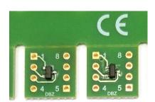
**Step 1:** Solder IC(s) to adapter PCB. Parts may be hand soldered or attached with IR or hot air reflow techniques.
