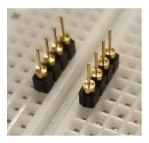
**Step 4:** Insert terminal strips into a breadboard or spare DIP socket to align pins.
