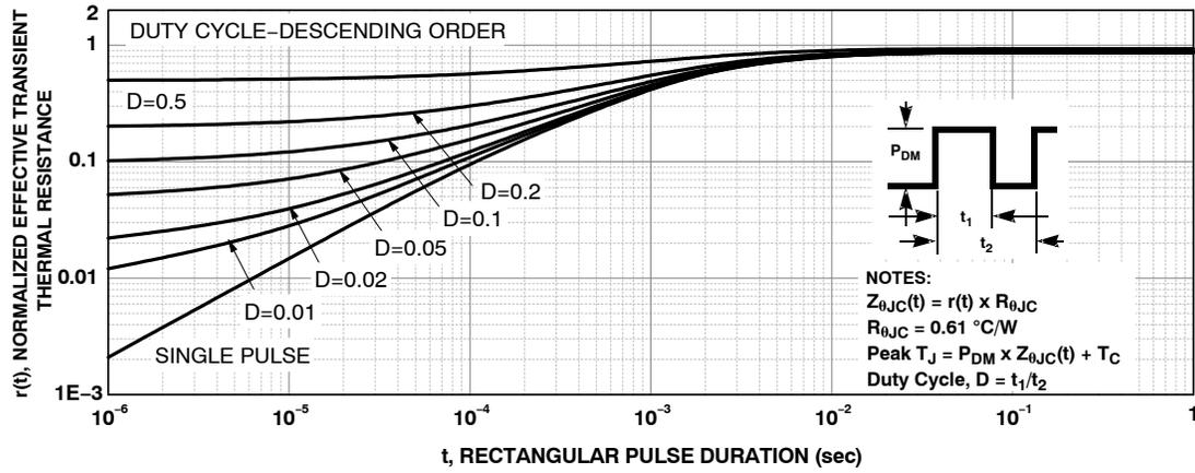
Figure 8. Junction-to-Case Transient Thermal Response Curve
