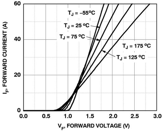
Figure 1. Forward Characteristics
