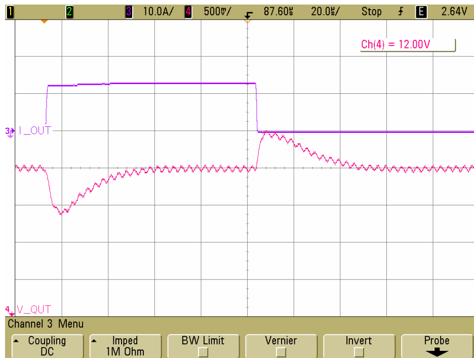
Figure 5. Load Transient Response (48Vin, 0A to 12Aout)
