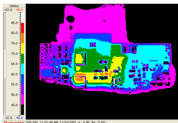
Figure 11. Temp Data (48Vin, 12Aout, 25°C, 200LFM airflow – back)
