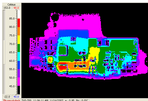
Figure 9. Temp Data (36Vin,12Aout, 25°C, 200LFM airflow – back)
