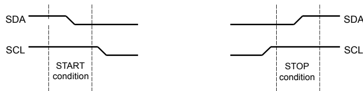
Figure 15-3. START and STOP Conditions
