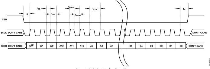
Figure 81. Serial Port Interface Timing Diagram
