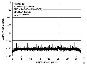
Figure 20. AD6655-150 Single-Tone FFT with  $f_{\text{IN}}$  = 30.3 MHz,  $f_{\text{NCO}}$  = 24 MHz
