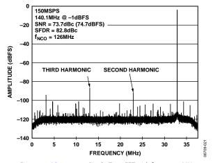
Figure 22. AD6655-150 Single-Tone FFT with  $f_{\text{IN}}$  = 140.1 MHz,  $f_{\text{NCO}}$  = 126 MHz
