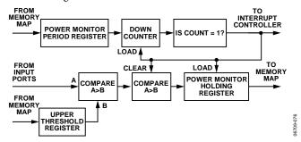
Figure 78. ADC Input Threshold Crossing Block Diagram
