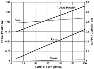
Figure 64. AD6655-150 Power and Current vs. Sample Rate
