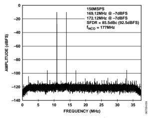
Figure 40. AD6655-150 Two Tone FFT with  $f_{\text{IN1}} = 169.12$  MHz,  $f_{\text{IN2}} = 172.12$  MHz,  $f_{\text{S}} = 150$  MSPS,  $f_{\text{NCO}} = 177$  MHz
