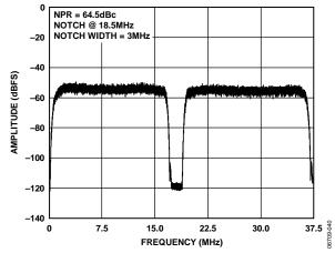
Figure 41. AD6655-150 Noise Power Ratio (NPR)
