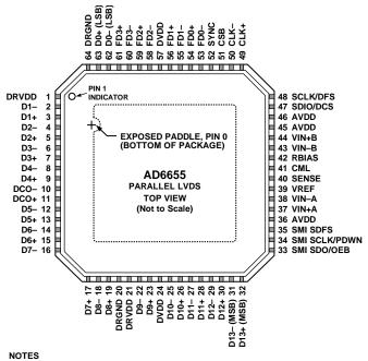
Figure 10. LFCSP Interleaved Parallel LVDS Pin Configuration (Top View)
