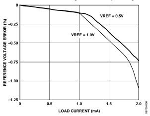
Figure 54. VREF Accuracy vs. Load
