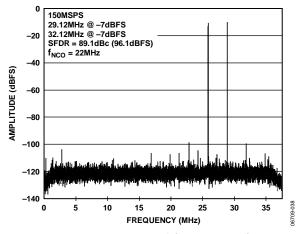
Figure 39. AD6655-150 Two-Tone FFT with  $f_{\text{IN1}} = 29.12$  MHz,  $f_{\text{IN2}} = 32.12$  MHz,  $f_{\text{S}} = 150$  MSPS,  $f_{\text{NCO}} = 22$  MHz
