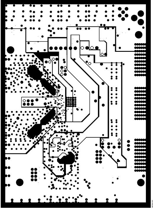
Figure 98. Evaluation Board Layout, Power Plane
