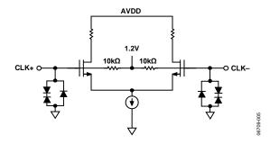
Figure 12. Equivalent Clock Input Circuit
