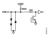
Figure 17. Equivalent CSB Input Circuit
