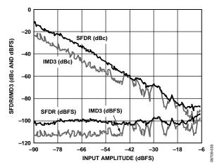
Figure 36. AD6655-150 Two-Tone SFDR/IMD3 vs. Input Amplitude ( $A_{IN}$ ) with  $f_{IN1}=29.12$  MHz,  $f_{IN2}=32.12$  MHz,  $f_{S}=150$  MSPS,  $f_{NCO}=22$  MHz
