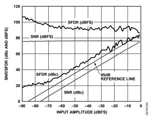
Figure 31. AD6655-150 Single-Tone SNR/SFDR vs. Input Amplitude (A<sub>IN</sub>) with  $f_{\rm IN}$  = 2.4 MHz,  $f_{\rm NCO}$  = 18.75 MHz
