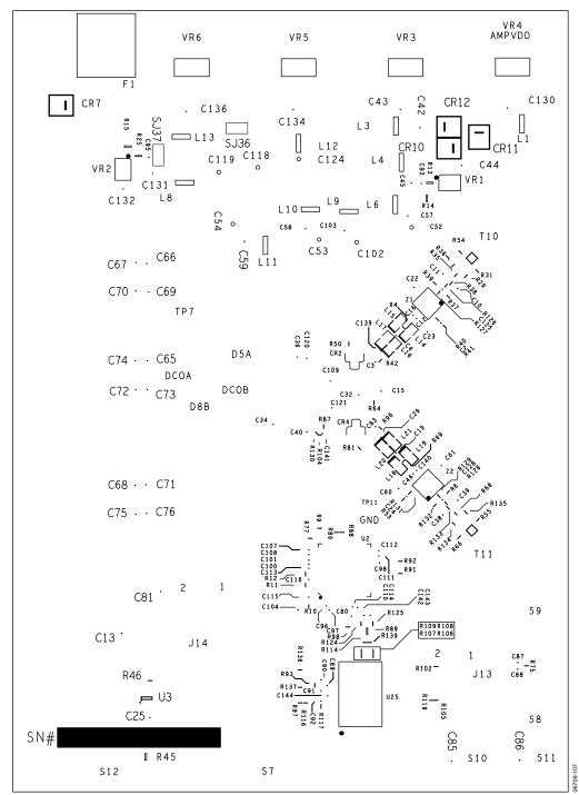
Figure 102. Evaluation Board Layout, Silkscreen, Secondary Side
