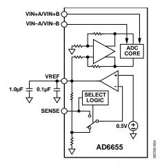
Figure 52. Internal Reference Configuration
