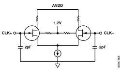
Figure 56. Equivalent Clock Input Circuit
