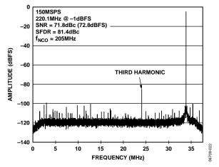
Figure 23. AD6655-150 Single-Tone FFT with  $f_{\rm IN}$  = 220.1 MHz,  $f_{\rm NCO}$  = 205 MHz
