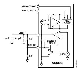
Figure 53. Programmable Reference Configuration
