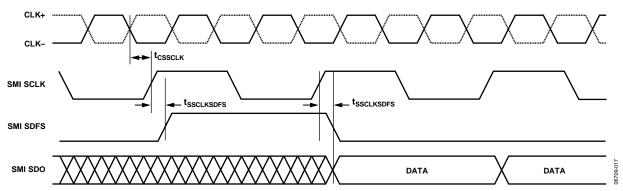
Figure 8. Signal Monitor SPORT Output Timing
