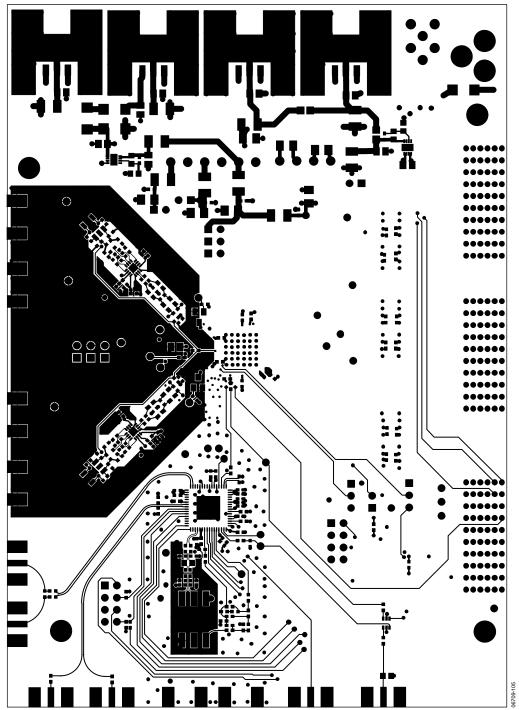
Figure 100. Evaluation Board Layout, Secondary Side (Mirrored Image)
