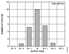
Figure 43. AD6655 Grounded Input Histogram
