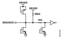
Figure 14. Equivalent SDIO/DCS Circuit or SMI SDFS Circuit
