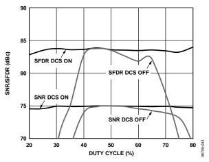
Figure 44. AD6655-150 SNR/SFDR vs. Duty Cycle with  $f_{\rm IN}$  = 30.3 MHz,  $f_{\rm NCO}$  = 45 MHz
