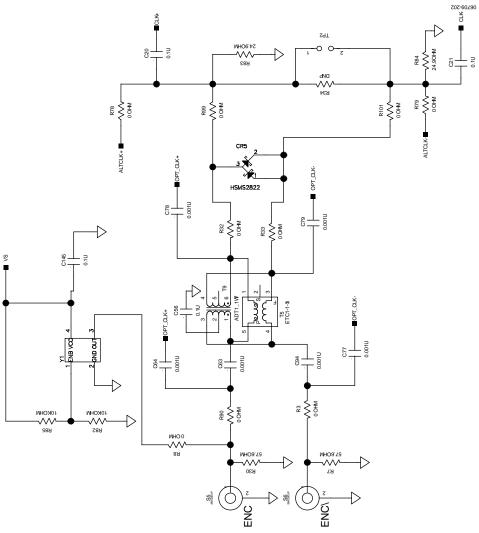
Figure 87. Evaluation Board Schematic, DUT Clock Input
