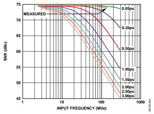
Figure 63. SNR vs. Input Frequency and Jitter
