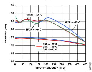
Figure 33. AD6655-125 Single-Tone SNR/SFDR vs. Input Frequency ( $f_{\rm IN}$ ) and Temperature with DRVDD = 1.8 V
