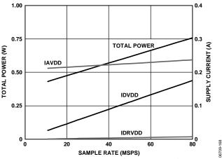
Figure 67. AD6655-80 Power and Current vs. Sample Rate
