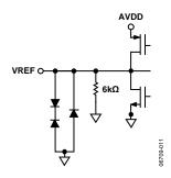
Figure 18. Equivalent VREF Circuit
