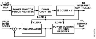
Figure 77. ADC Input RMS Magnitude Monitoring Block Diagram
