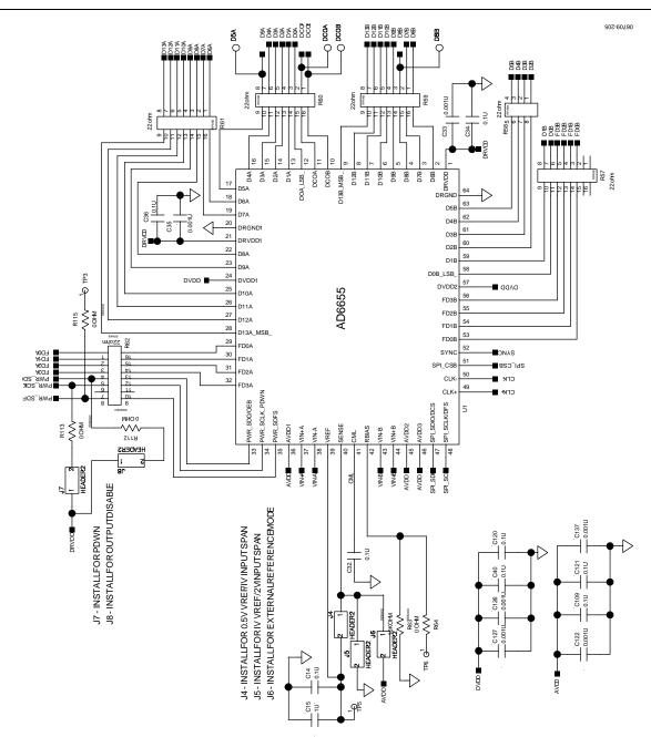
Figure 90. Evaluation Board Schematic, DUT
