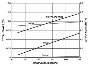
Figure 65. AD6655-125 Power and Current vs. Sample Rate
