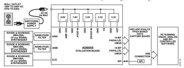
Figure 84. Evaluation Board Connection
