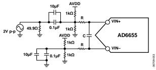
Figure 51. Single-Ended Input Configuration
