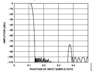
Figure 74. Half-Band Filter and FIR Filter Composite Response
