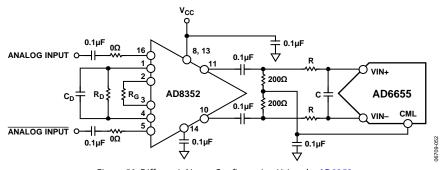
Figure 50. Differential Input Configuration Using the AD8352
