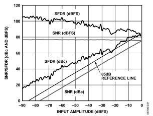
Figure 32. AD6655-150 Single-Tone SNR/SFDR vs. Input Amplitude (A<sub>IN</sub>) with  $f_{\rm IN}$  = 98.12 MHz,  $f_{\rm NCO}$  = 100.49 MHz
