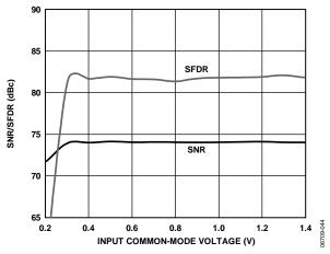
Figure 45. AD6655-150 SNR/SFDR vs. Input Common Mode (V<sub>CM</sub>) with  $f_{IN}=30.3~MHz,\,f_{NCO}=45~MHz$
