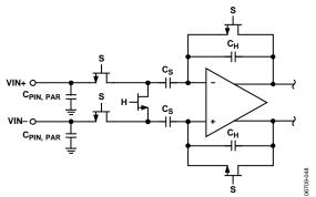
Figure 46. Switched-Capacitor SHA Input
