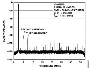
Figure 19. AD6655-150 Single-Tone FFT with  $f_{\text{IN}}$  = 2.4 MHz,  $f_{\text{NCO}}$  = 18.75 MHz
