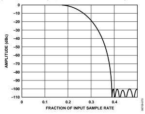
Figure 72. Half-Band Filter Low-Pass Response
