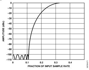
Figure 73. Half-Band Filter High-Pass Response
