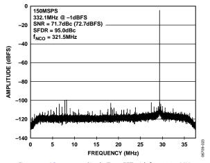
Figure 24. AD6655-150 Single-Tone FFT with  $f_{\text{IN}}$  = 332.1 MHz,  $f_{\text{NCO}}$  = 321.5 MHz
