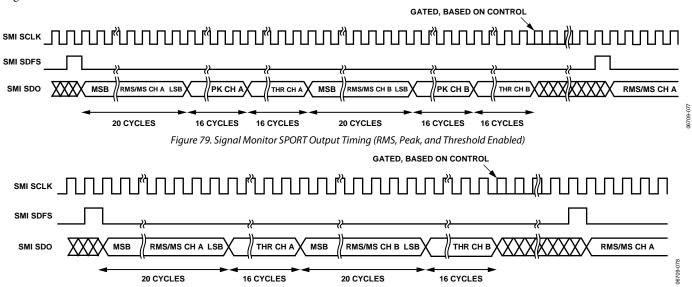
Figure 80. Signal Monitor SPORT Output Timing (RMS and Threshold Enabled)
