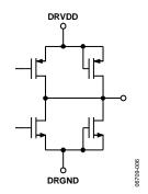
Figure 13. Equivalent Digital Output Circuit
