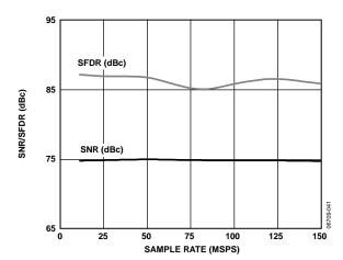
Figure 42. AD6655-150 Single-Tone SNR/SFDR vs. Sample Rate ( $f_s$ ) with  $f_{\rm IN}$  = 2.3 MHz
