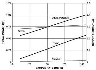
Figure 66. AD6655-105 Power and Current vs. Sample Rate
