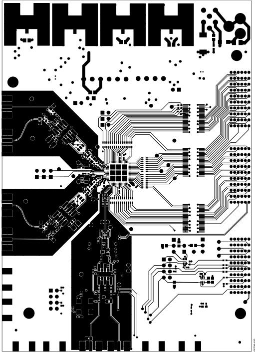
Figure 95. Evaluation Board Layout, Primary Side
