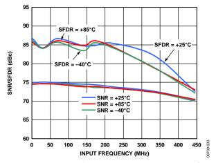
Figure 34. AD6655-125 Single-Tone SNR/SFDR vs. Input Frequency ( $f_{\rm IN}$ ) and Temperature with DRVDD = 3.3 V
