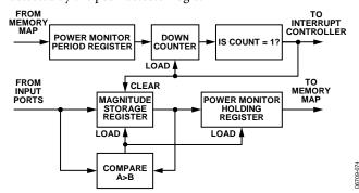
Figure 76. ADC Input Peak Detector Block Diagram
