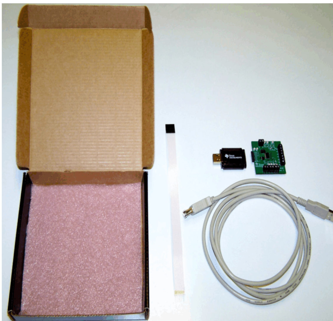
Figure 1. Typical Hardware Included with the AMC80EVM Kit
