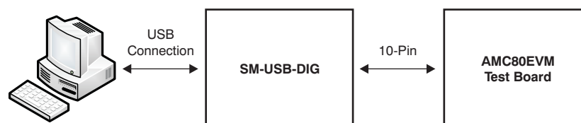
Figure 2. AMC80EVM Hardware Setup
