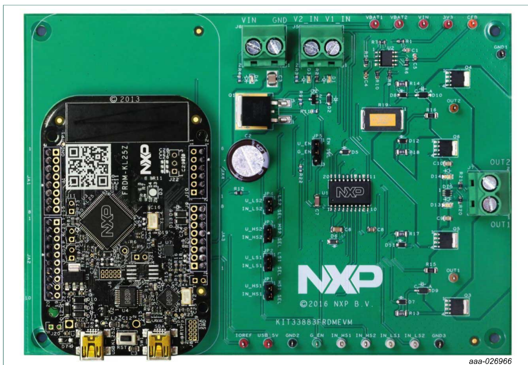
Figure 1. KIT33883FRDM-EVM with FRDM-KL25Z Freedom Development Platform
