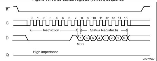
Figure 11. Write Status register (WRSR) sequence
