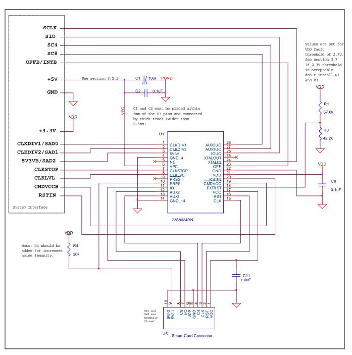
Figure 3-1: Typical Schematic using the 73S8024RN for NDS Applications
