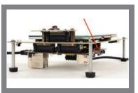
Insert the microSD card into the AM572x EVM processor board.
