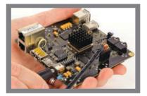
Connect the supplied power cable to the processor board as shown (for simplicity only the processor board is shown). Connect the 12-volt power supply cable to an AC power source.
