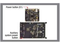
To turn on, press and release power button (S1) or auxiliary power button. To turn off, press and hold the same button for 15 sec. Do not unplug the power supply to turn off the board, as it may cause damage.
