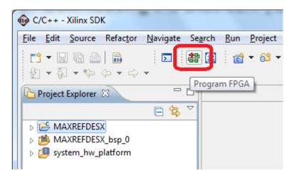
The Program FPGA dialog box appears. From here, an FPGA bitstream (.BIT) file is selected as well as an FPGA bmm (.BMM) file. Be sure to select the .BIT file and the .BMM by using the paths below.
