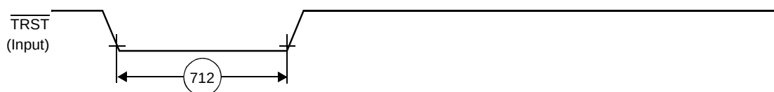
Figure 29. \overline{\text{TRST}} Timing Diagram
