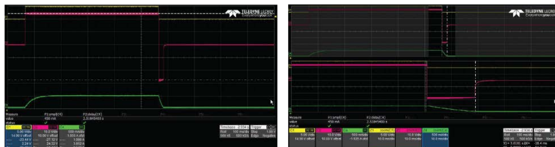
Figure 11. ITS4880 with fast demag (A - V CLAMP , B - t DEMAG ).
