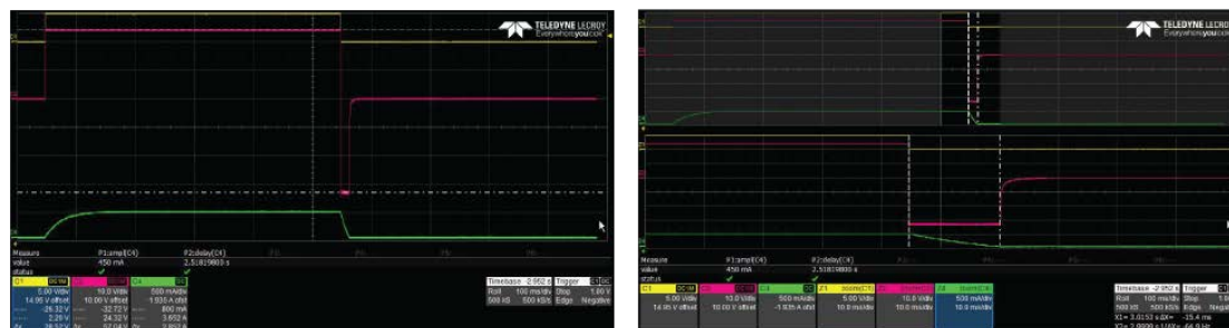
Figure 10. MAX14912 with fast demag (A - V CLAMP , B - t DEMAG ).
