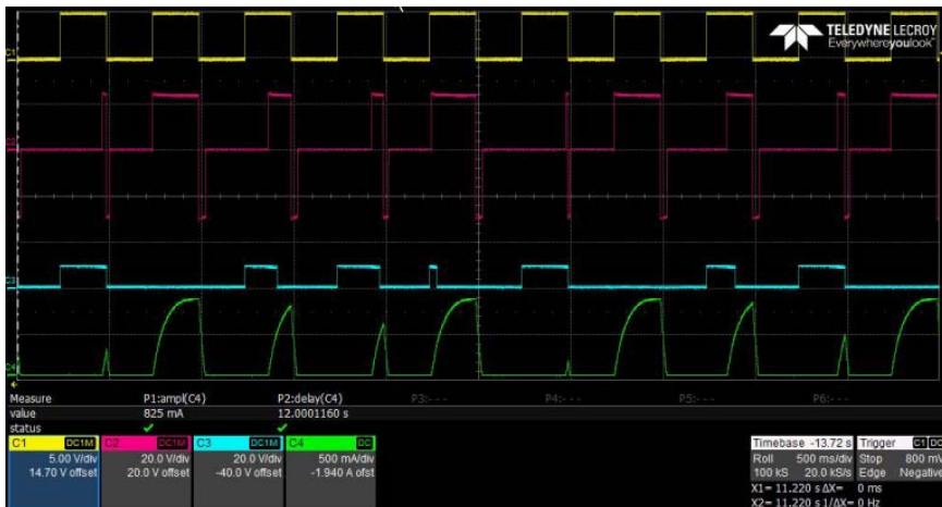
Figure 14b. ITS4880R switching inductor loads for all eight channels simultaneously.
