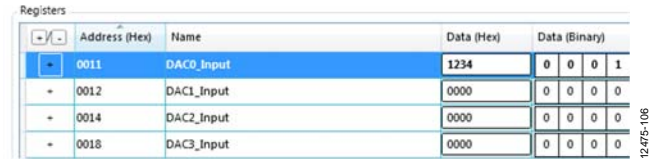
Figure 6. AD5696R Memory Map with Unapplied Changes in the DAC0_Input Register
