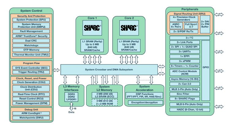
Figure 2. A block diagram of the dual SHARC core ADSP-21584 digital signal processor from Analog Devices.
